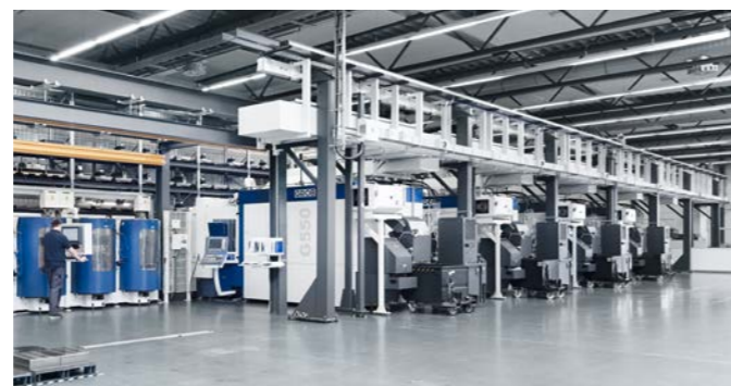
Fully automatic milling center with 5-axis milling machines
