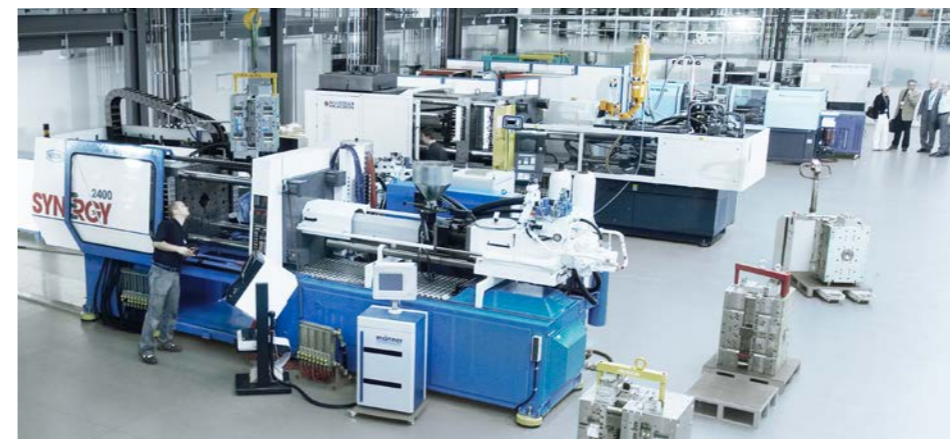
Test Center with injection molding machines from 75 to 500 tons
