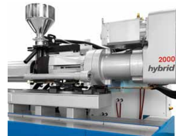
Hybrid high-performance injection unit
