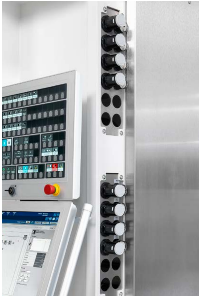
All pneumatic valves can be adjusted with the safety cover closed
