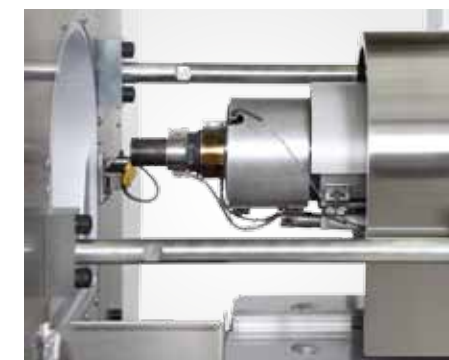
Optimized process control thanks to actively controlled nozzle needle valve
