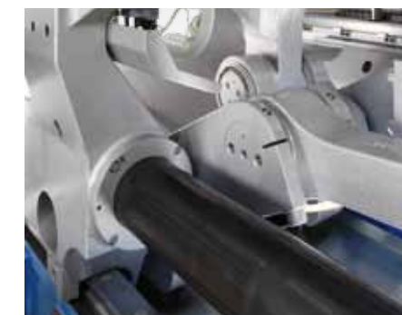
Transfer of force through centrally inclined 5-point toggle lever
