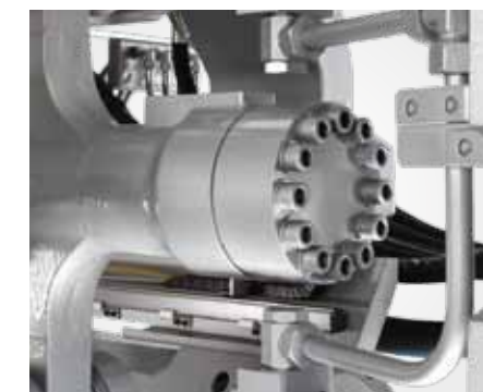
Reduced footprint thanks to inward-facing closing cylinder
