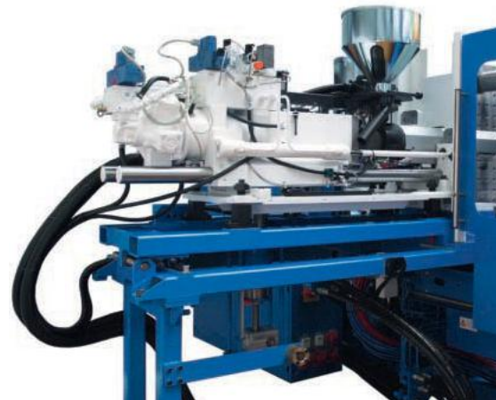
The second injection unit is firmly connected to the base frame in L-shape
