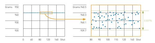
Shot weight consistency 0.037%, based on the example of 20 liter buckets in 2 cavities with a shot weight of 940 g [PE]
