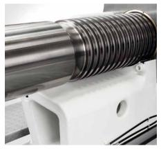
Molds are protected in every position thanks to the guided tiebars.
