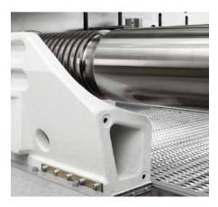
The force flow- and weight-optimized sliding shoes ensure that the moving platens are quided securely.
