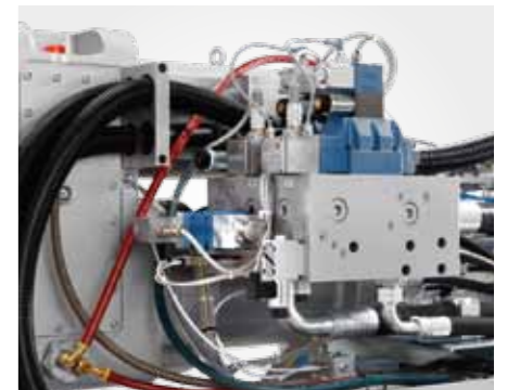
Auxiliary mold control: extremely dynamic thanks to state-of-the-art valve technology
