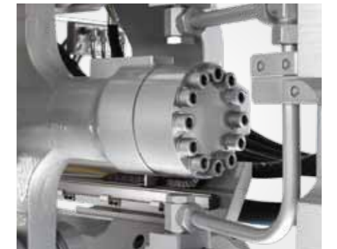
Reduced footprint thanks to inward-facing closing cylinder
