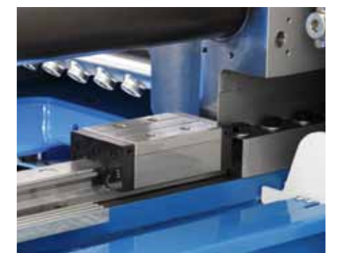
EVOS can be optionally equipped with a freely movable support for stack molds.
