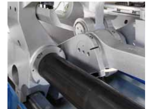
Transfer of force through centrally inclined 5-point toggle lever
