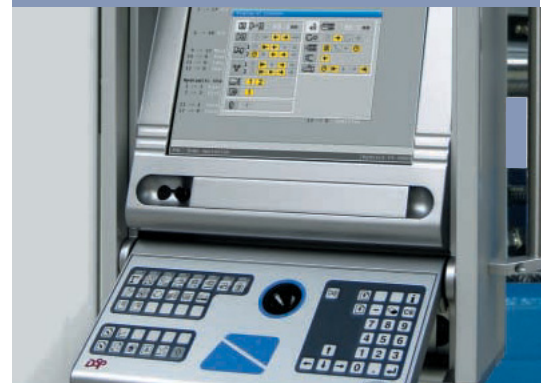
New operating unit with integrated sequence display
