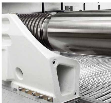
The force flow- and weight-optimized sliding shoes ensure that the moving platens are guided securely.
