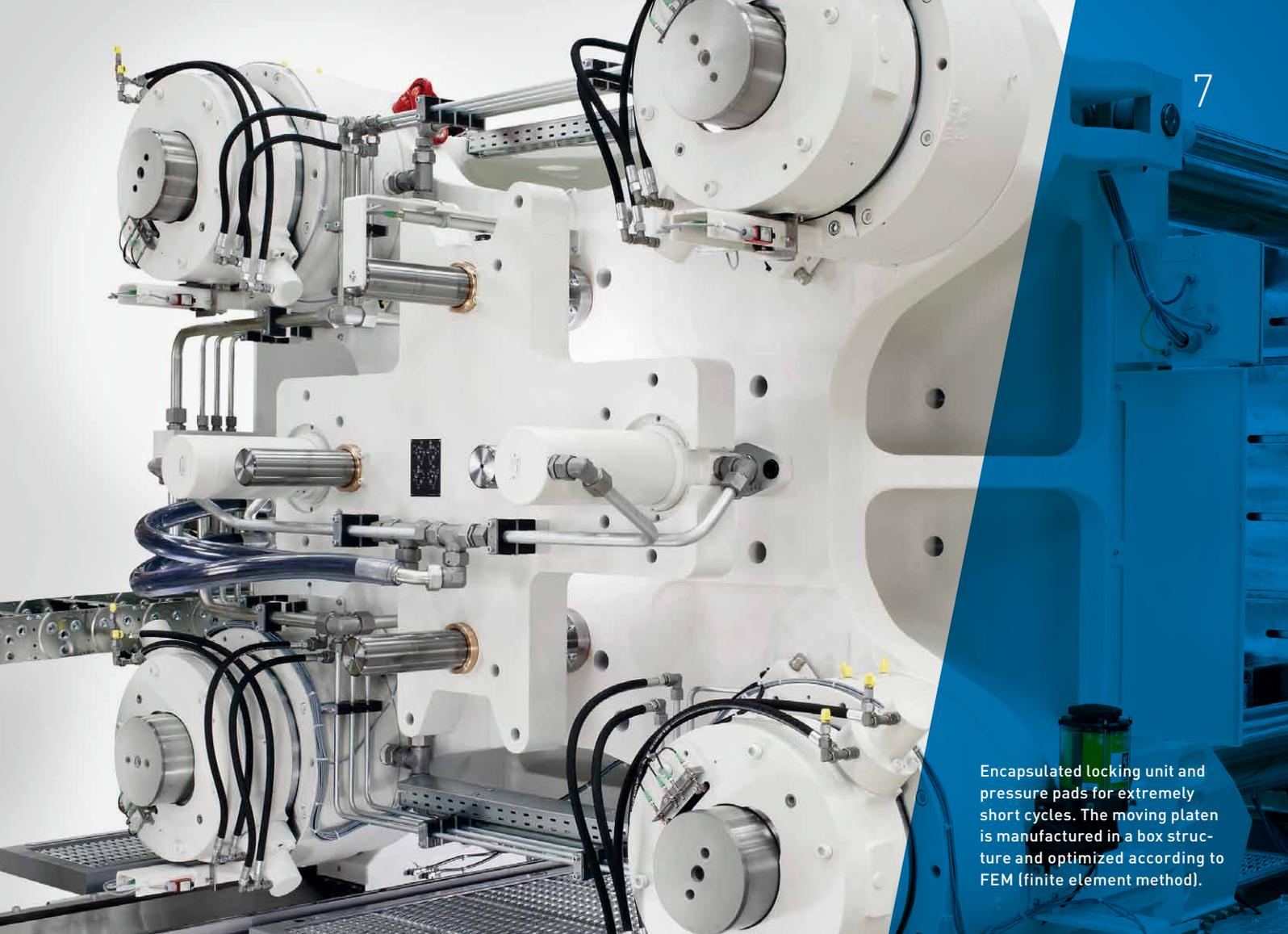
Encapsulated locking unit and pressure pads for extremely short cycles. The moving platen is manufactured in a box structure and optimized according to FEM (finite element method).
