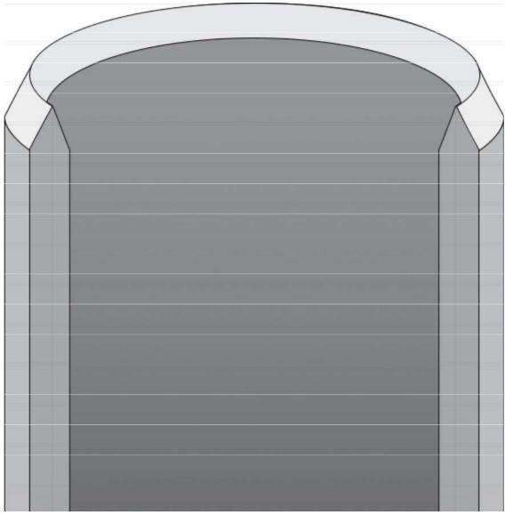
The middle edge is achieved by tapering the outside and inside diameter which yields a cutting edge approximately in the middle of the punch wall.
